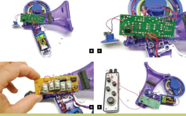
Figs. B and C: Search the circuit board for the audio generation IC, which is often a black blob "gumdrop." Fig. D: The pitch resistor is usually the resistor closest to the audio generation IC, often on the back.
