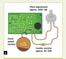
Fig. A: Replace the clock speed (aka pitch) resistor with a potentiometer and a limiting resistor.
