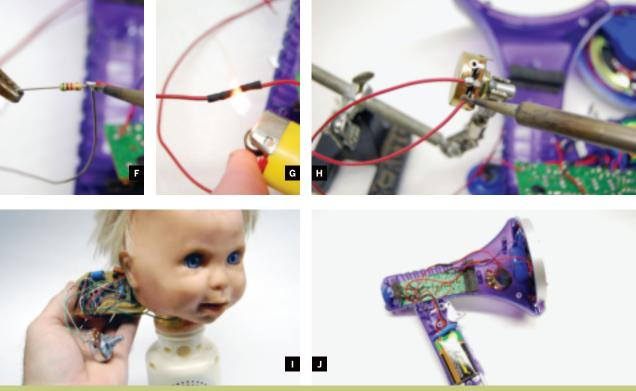
Fig. F: Wire up a limiting resistor to keep the pitch from going too high. Fig. G: Shrink a 1" piece of heatshrink tubing over the resistor. Fig. H: Wire up your potentiometer.
